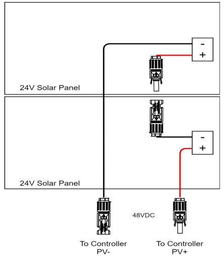
**STEP 9:** Once the batteries and solar panels are all connected and wired to the Large Green Connector, Disconnect PV+ wire and plug the connector to the MPPT Solar Controller until the connector latches click into place. The Battery Charging LED should light up for about 60 seconds. Now connect PV+ to the green connector.
