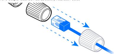
Ø3.3~4.5 mm (Ø0.13~0.18") Ø4.5~5.5 mm (Ø0.18~0.22") Ø5.5~6.5 mm (Ø0.22~0.26")
