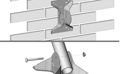
Install the pole to the base using pivot bolt
